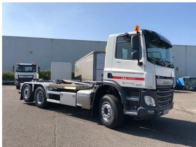
DAF CF 450 FAN 6X2 axle with HYVA Loader 20-53-S
